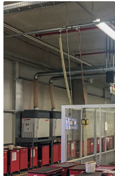
VACUMAT for aspiration at a workplace
