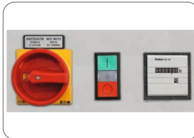
Control panel with operating hour meter
